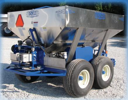
Heavy Duty Rectangular Steel Tubing Frame, with Heavy Duty Corner Braces
