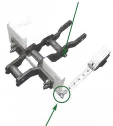
5/8" thick, long wearing UHMW paddles are mounted with stainless bolts.
